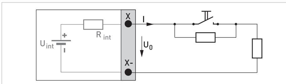
Figure 4-23: Control input active  $C_N$  according to NAMUR EN 60947-5-6
