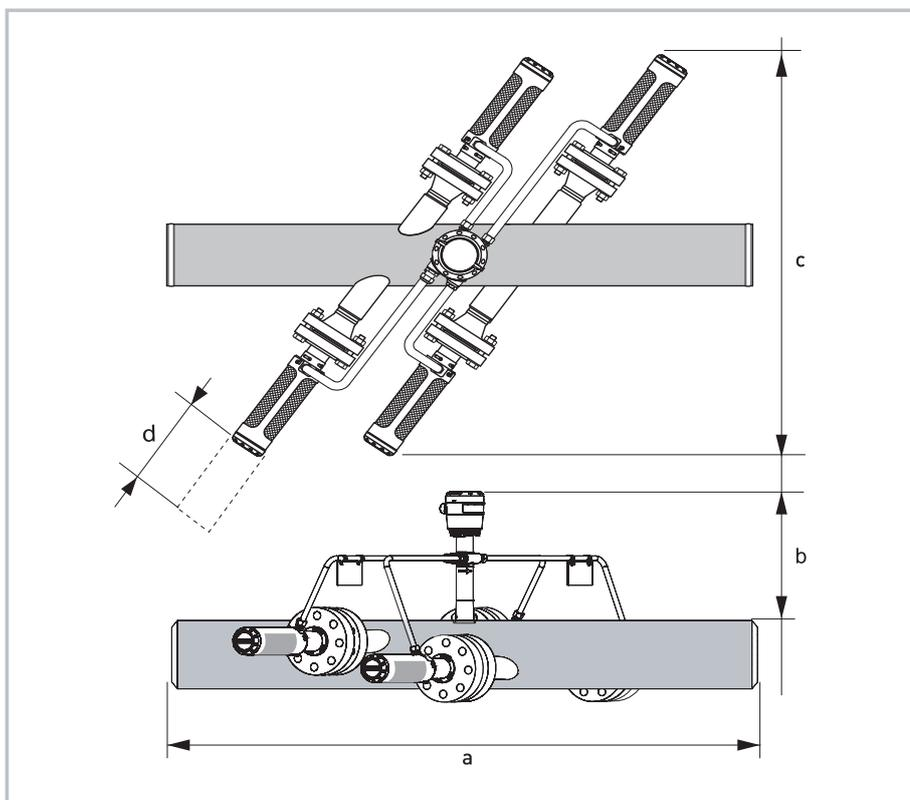
Figure 8-2: Top and front view of the OPTISONIC 8000
