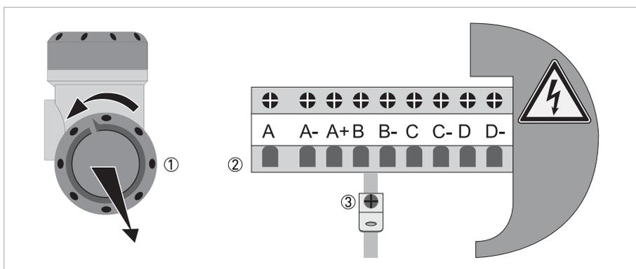
Figure 4-6: Terminal compartment for inputs and outputs
