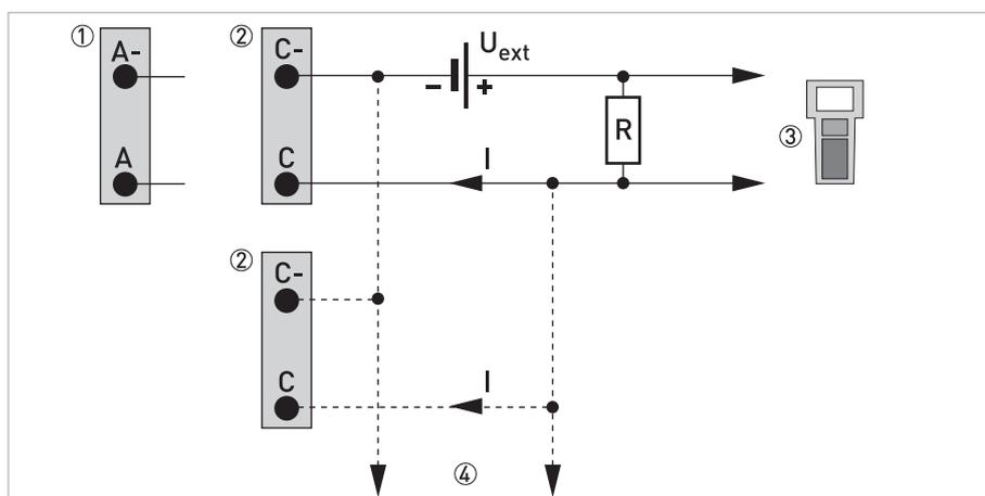
Figure 4-34: HART<sup>®</sup> connection passive ( $I_p$ )
