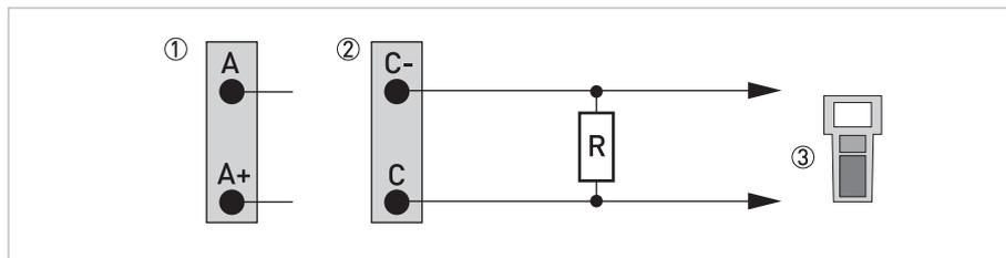
Figure 4-33: HART<sup>®</sup> connection active ( $I_a$ )
