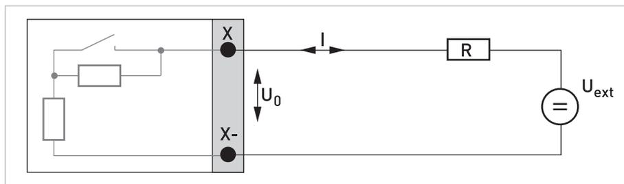
Figure 4-17: Pulse/frequency output passive P<sub>N</sub> according to NAMUR EN 60947-5-6
