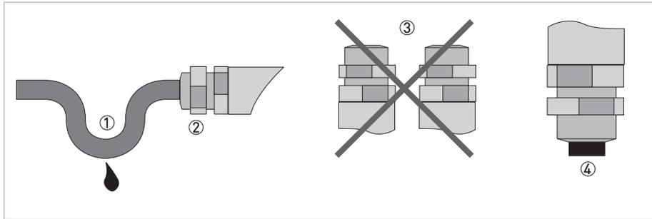
Figure 4-7: Protect housing from dust and water
