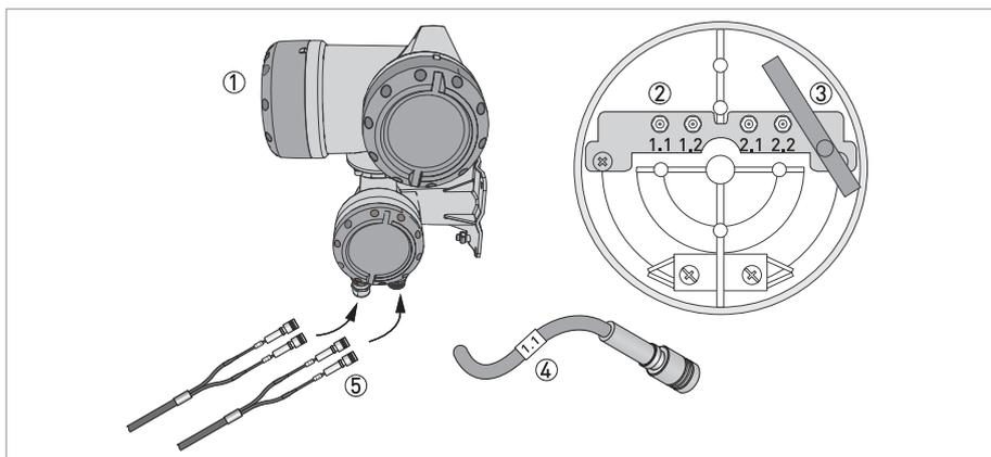
Figure 4-1: Connection of signal cable to signal converter
