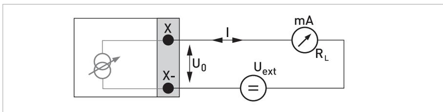
Figure 4-27: Current output passive  $I_p$  Ex i
