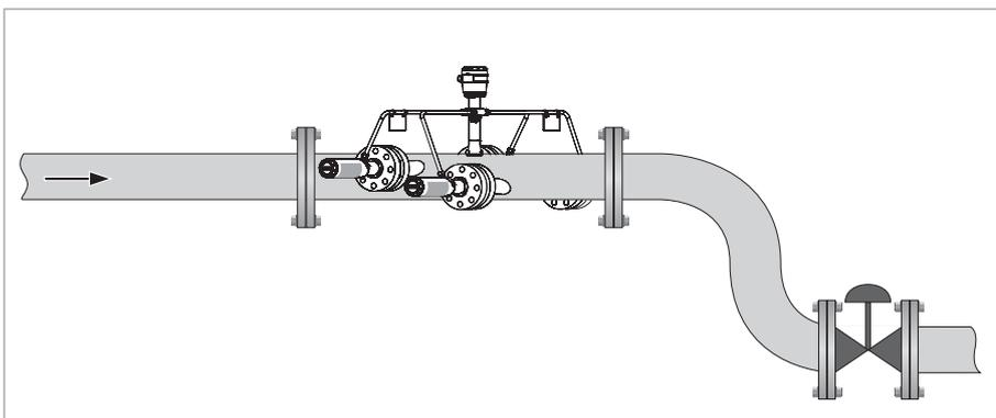
Figure 3-8: Recommended installation of the control valve
