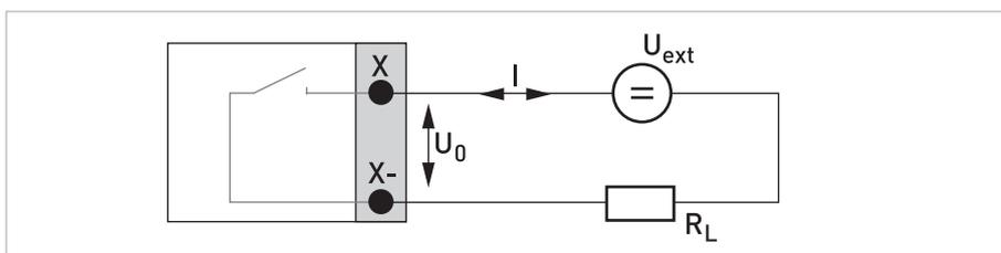
Figure 4-19: Status output / limit switch passive  $S_p$
