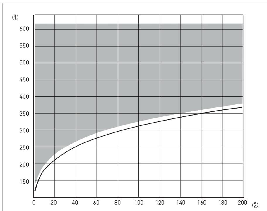
Figure 1-1: Steam saturation curve
