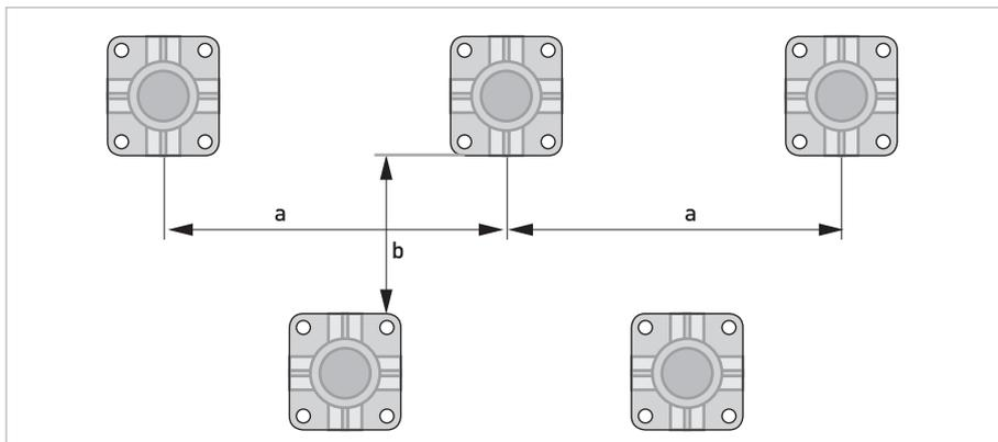
Figure 3-12: Mounting multiple devices next to each other
