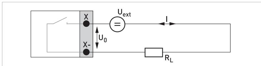
Figure 4-11: Status output / limit switch passive  $S_p$ **Control input passive, basic I/Os**
