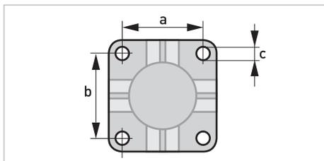
Figure 8-4: Dimensions for mounting plate of field housing
