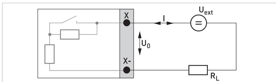
Figure 4-28: Pulse/frequency output passive P<sub>N</sub> according to NAMUR EN 60947-5-6 Ex i
