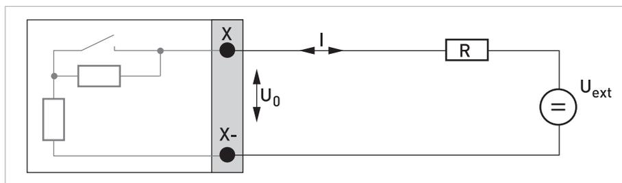
Figure 4-20: Status output / limit switch  $S_N$  according to NAMUR EN 60947-5-6
