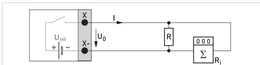
Figure 4-15: Pulse/frequency output active  $P_a$
