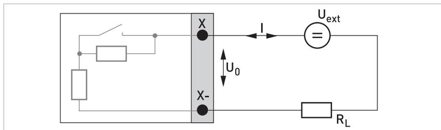
Figure 4-29: Status output / limit switch  $S_N$  according to NAMUR EN 60947-5-6 Ex i
