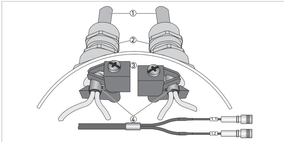
Figure 4-2: Clamp the cables on the shielding bush
