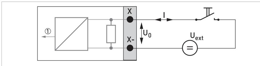
Figure 4-30: Control input passive  $C_p$  Ex i
