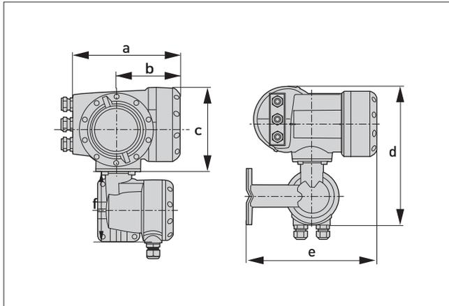
Figure 8-3: Field housing (F) - remote version.
