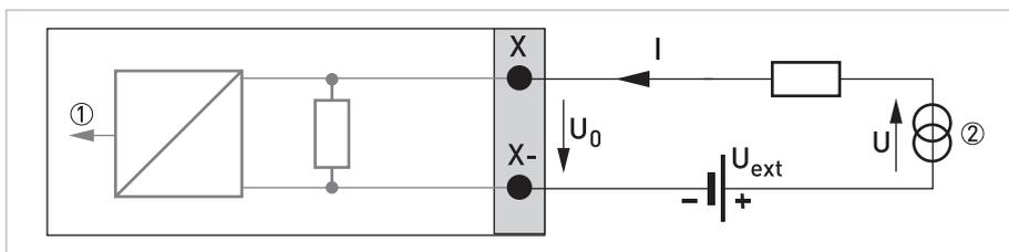
Figure 4-25: Current input passive  $IIn_p$
