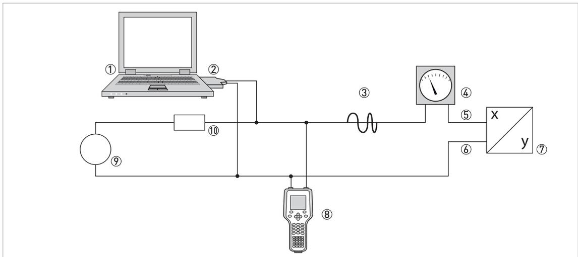
**Figure 9-1: Point-to-Point connection**
