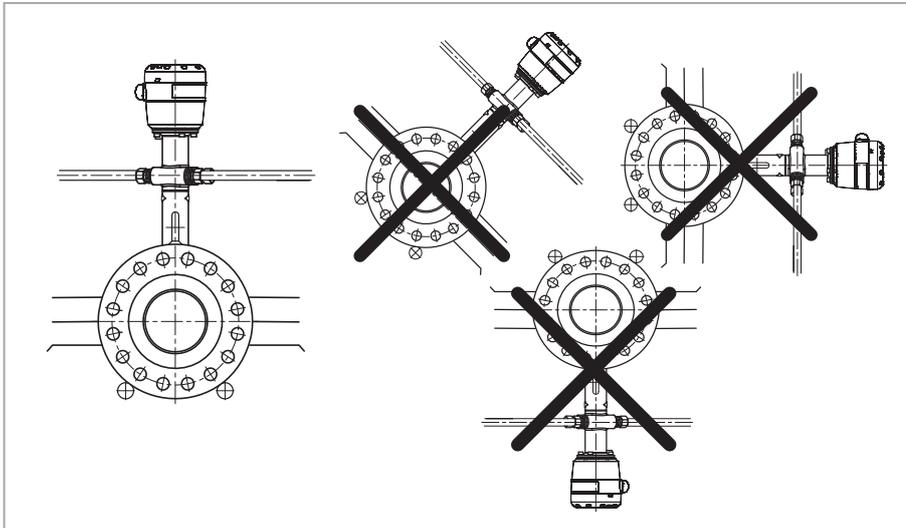
Figure 3-6: Mounting position
