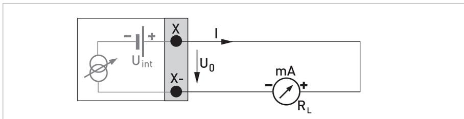
Figure 4-26: Current output active  $I_a$  Ex i
