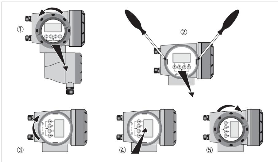
Figure 3-13: Turning the display of the field housing version
