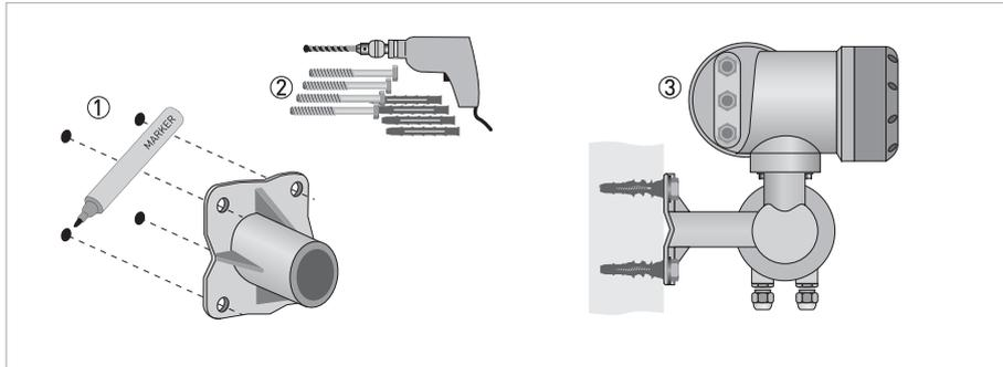
Figure 3-11: Wall mounting of the field housing
