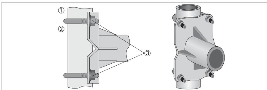
Figure 3-10: Pipe mounting of the field housing
